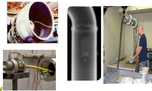
RADIOGRAPHY TESTING OF AIRCRAFT ENGINE
